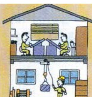
Factory building with an office on the upper level(The building does not shake.)
